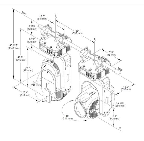
POSITIONING:SPACING:WEIGHT:Can be mounted in any orientation.Hangs on 30 inch (762 mm) centers.171 lbs (77 Kg) without hooks
