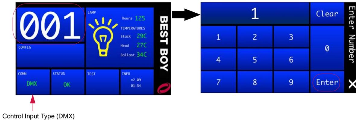
Figure 2-15: Setting Starting Address (DMX Control)
