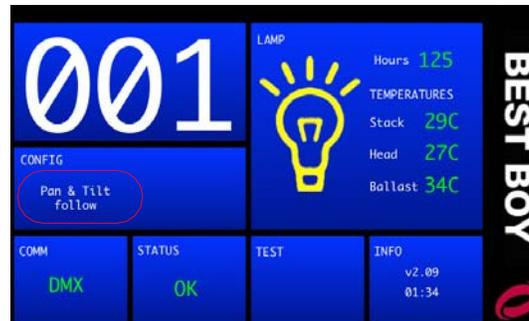
Note that the Followspot Controller device does not need to be connected in order to enable followspot control on the luminaire. If there is no FSC connected while in Followspot mode, the selected mechanisms will simply ignore DMX until Followspot mode is exited.
