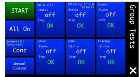
**Group Tests Screen** - Allows multiple luminaires to be tested when daisy-chained together.
