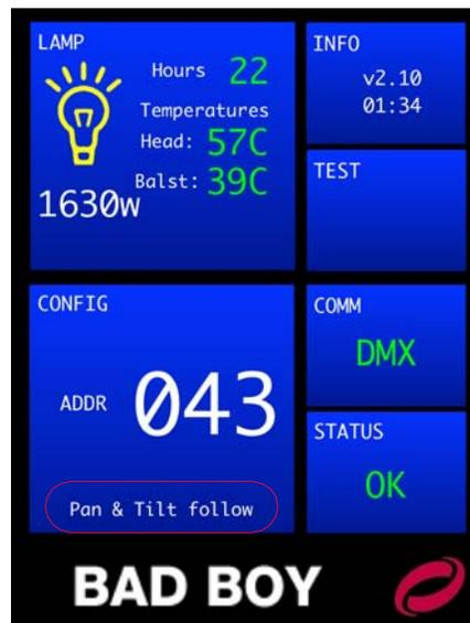
Note that the Followspot Controller device does not need to be connected in order to enable followspot control on the luminaire. If there is no FSC connected while in Followspot mode, the selected mechanisms will simply ignore DMX until Followspot mode is exited.
