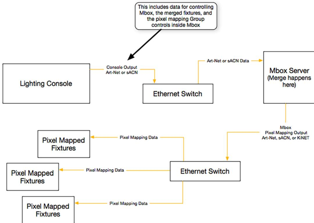
Figure 1: Example Merge Hardware I/O Diagram 1
