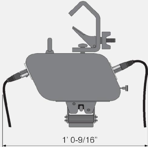
KABUKI G2 is the Gerriets system for reliably dropping any type of curtain in a fraction of a second. The newly developed, electronically controlled, and extremely quick KABUKI G2 system allows load ratings up to 22 lbs. per release unit. That means 100 % higher load ratings than previous systems. A LED integrated into the bottom of the release unit is now standard. This added feature gives a visual confirmation from below that the unit is ready to be fired.
