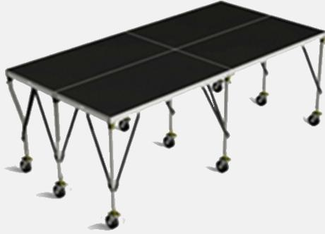
PRG Rolling Stage is a flexible, portable stage that offers strength and durability and is also quick to assemble. The Rolling Stage is engineered for safe, efficient and rapid deployment and is easily repositioned and reconfigured. The design is based on a standard 4'x8' (1.22m x 2.44m) size.
