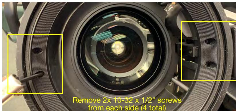
Figure 3-38: Removing the Light Shield Assembly
