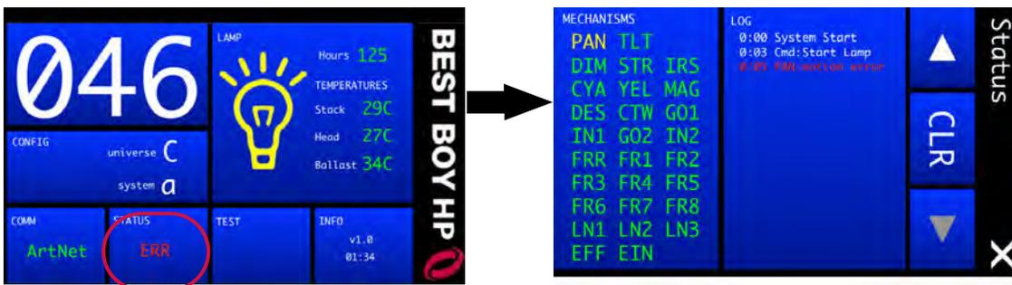
The Status screen will indicate which specific mechanisms, if any, have errors. It also provides a log of systems activity. The Status screen operates as follows:
