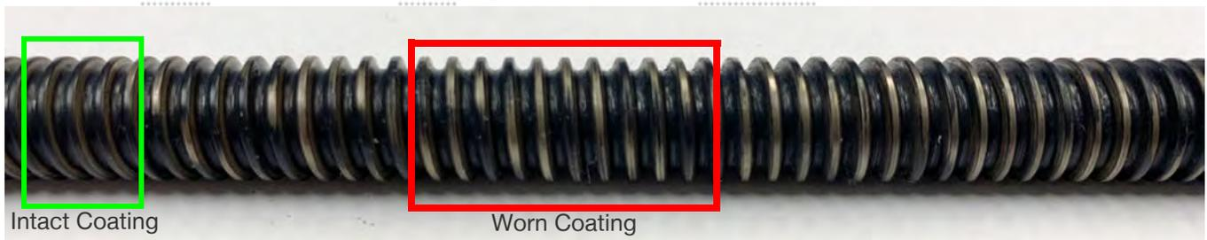
Figure 3-36: Lead Screw with Coating Worn from Threads
