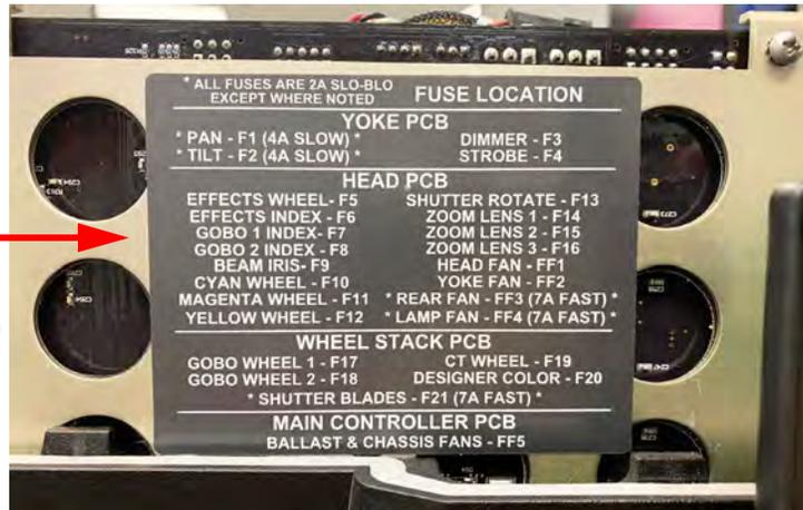
Figure 2-2: Fuse Map Location on Head PCB Bracket
