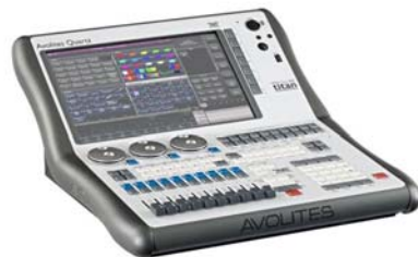
Quartz +16 Universes of DMX Processing +4 DMX Ports
