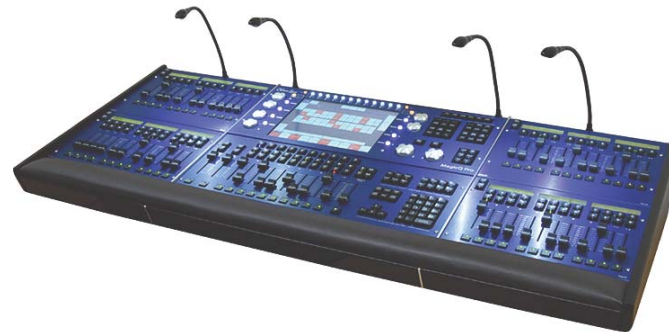
MagicQ MQ300 Pro 2014 +64 Universes of DMX Processing +4 DMX Ports
