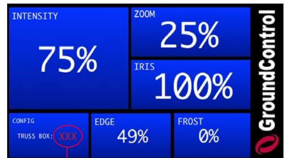
Truss Box Error Indication
