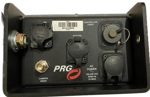
*New connector panel with outdoor-rated connectors.*
