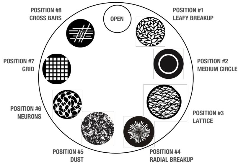
This chart represents the PRG standard gobo wheel configuration for the VL2600 Profile luminaire.
